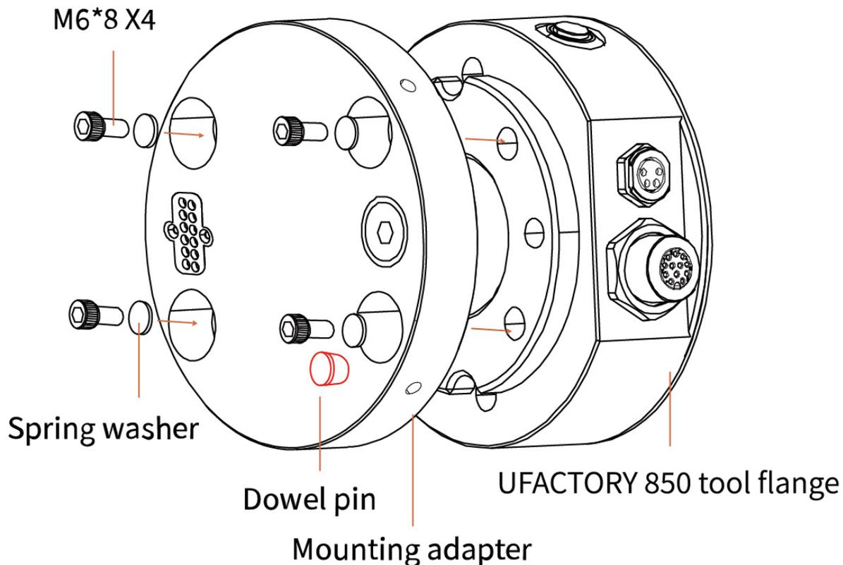
3) Install the 6 Axis Force Torque Sensor on the Mounting Flange using 4 M3\*8 screws (spring washer must be used together).
